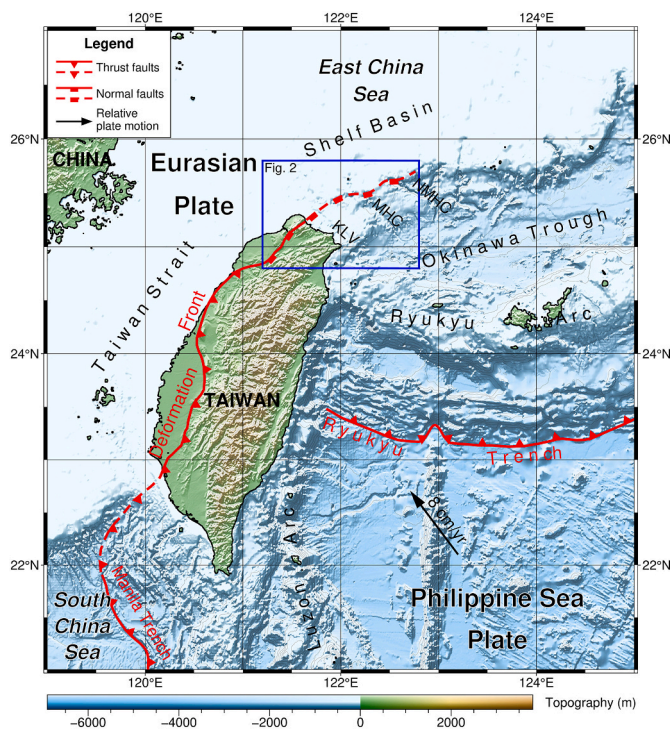
Fig. 1. Tectonic and topographic/bathymetric map of Taiwan and adjacent areas. In northern Taiwan and its offshore area, fault behavior changes gradually from thrust faults in the south to normal faults in the north. The deformation front, Manila Trench and Ryukyu Trench are inferred from previous studies (Sibuet and Hsu, 2004; Yu, 2005; Lin et al., 2008; Hsu et al., 2013). The convergence rate (8 cm/yr) is proposed by Yu et al. (1997). The red dashed lines indicate faults or trenches. The blue rectangle indicates our study area. NMHC: North Mienhua Canyon, MHC: Mienhua Canyon, and KLV: Keelung Valley. (For interpretation of the references to colour in this figure legend, the reader is referred to the web version of this article.)
